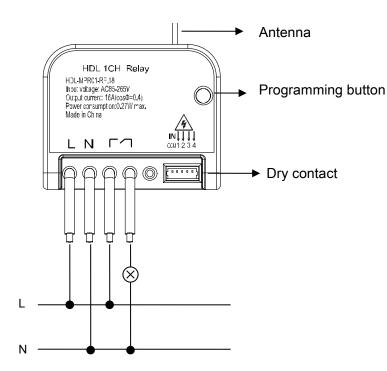
Programming button: if it is working properly, the green light will flicker, press the button three times continuously, the green light will flicker quickly, enters the wireless setup mode (the gateway should enter the setup mode at the same time, so that can set the wireless parameters for it)
