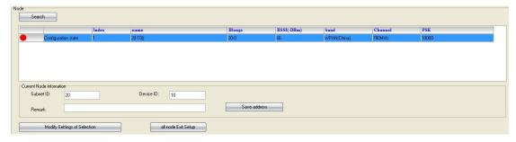
6- Click 'Modify Setting of Selection', then all its wireless parameters will follow the gateway's (Band, Frequency and PSK).
