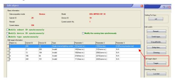
Can set each channel's controlled targets, the target's range is 1~20.
