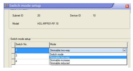
Each channel can set the mode **Switch mode**: on/off control
