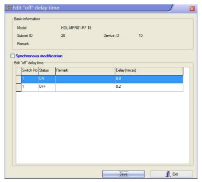
Only the "Mechanic switch" switch type has the delay time.
