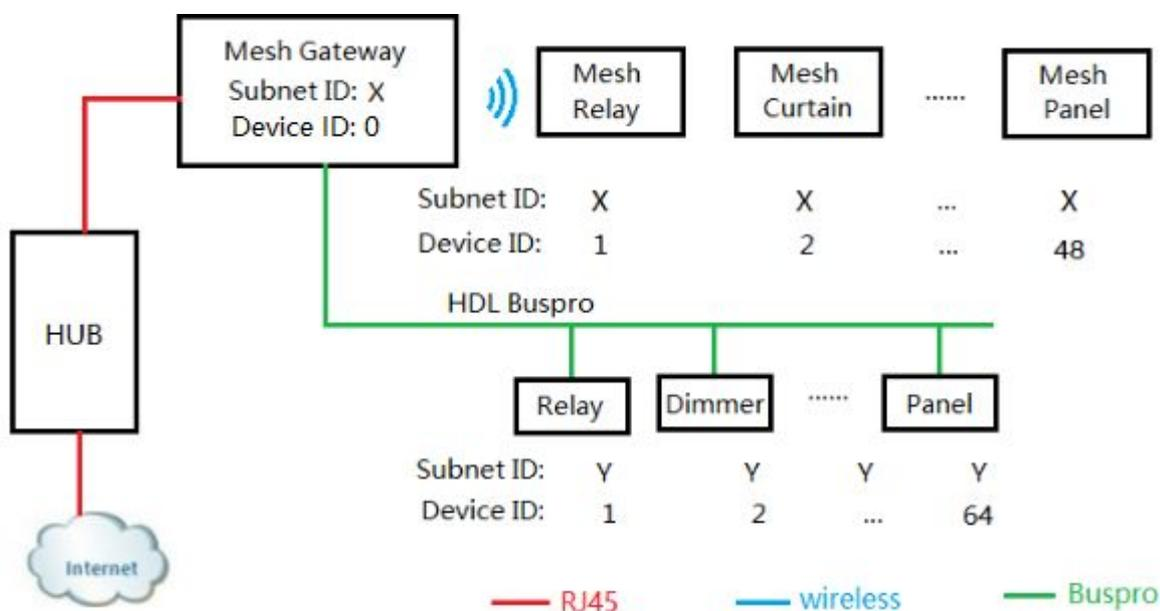
1) The Wireless Gateway is considered as a two port IP module, one port for Wireless System and the other for Wired System
