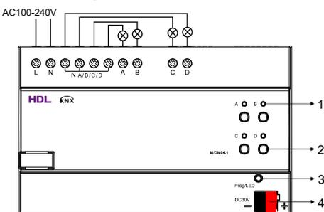
Take the connection of KNX 4CH 1.5A MOSFET Dimming Actuator as an example
